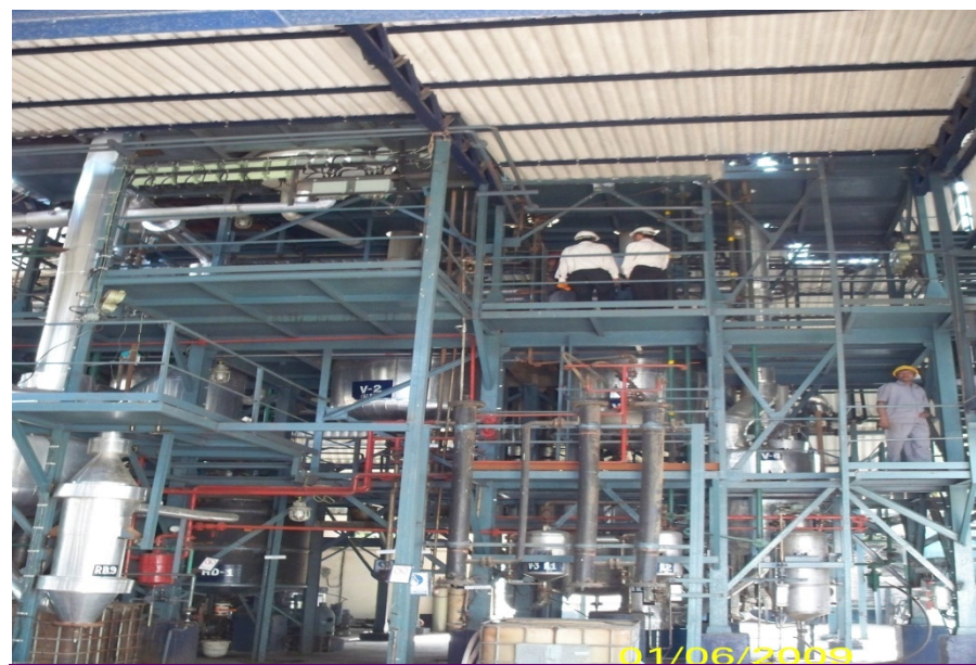
Semi-commercial plant(350 tpa) for production of vinyl esters at MEHIK Chemicals Pvt. Ltd, Thane
